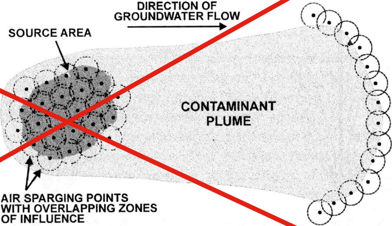
Air sparging point locations in a source area and in a curtain configuration.
