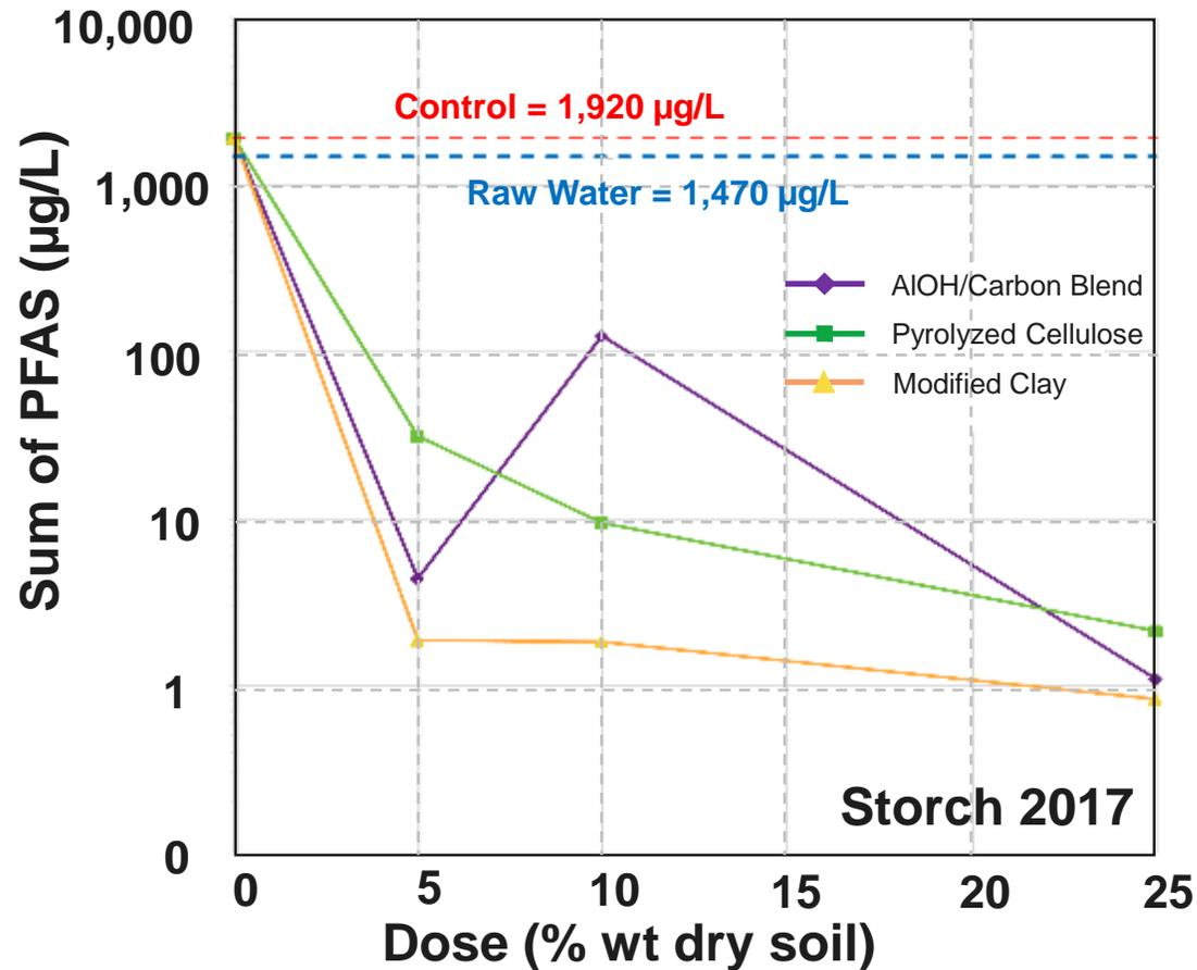
PFAS removal from supernatant in a soil/GW/adsorbent slurry at different % dry soil weight doses.
